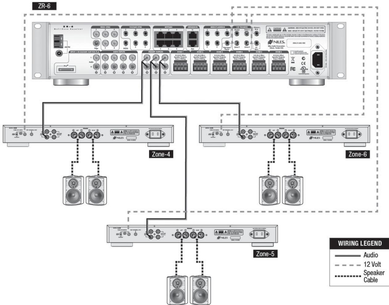
Figure 9. ZR-6 MultiZone Receiver with external amplifiers in zones 4, 5, 6
