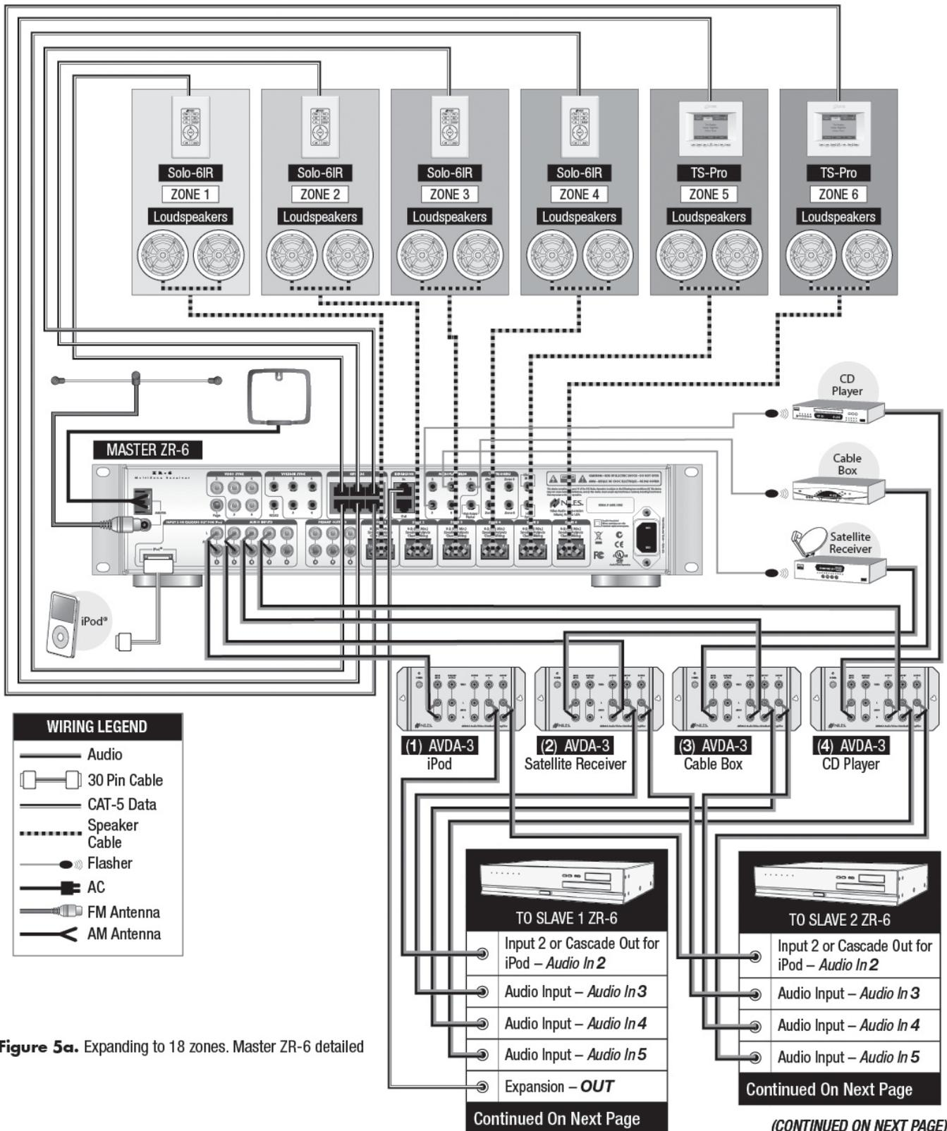
Figure 5a. Expanding to 18 zones. Master ZR-6 detailed
