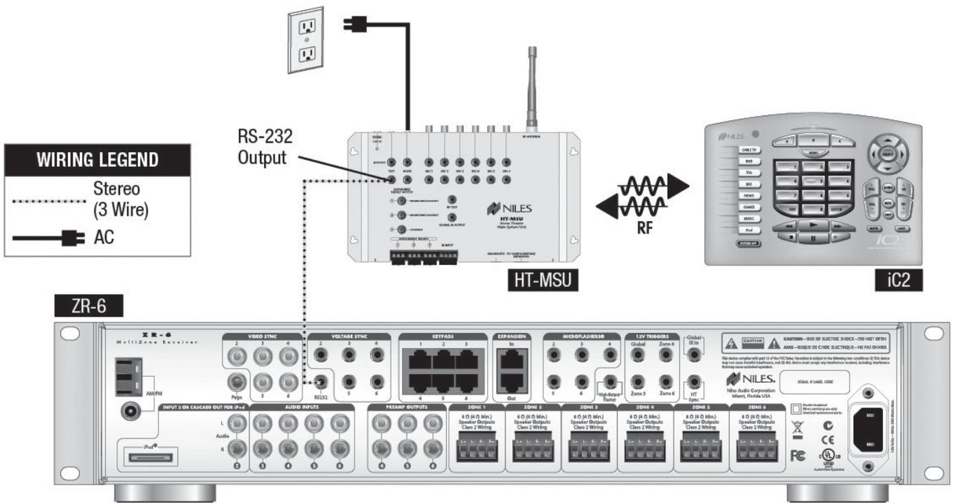
**Figure 7.** Connecting an external RS-232 control system
