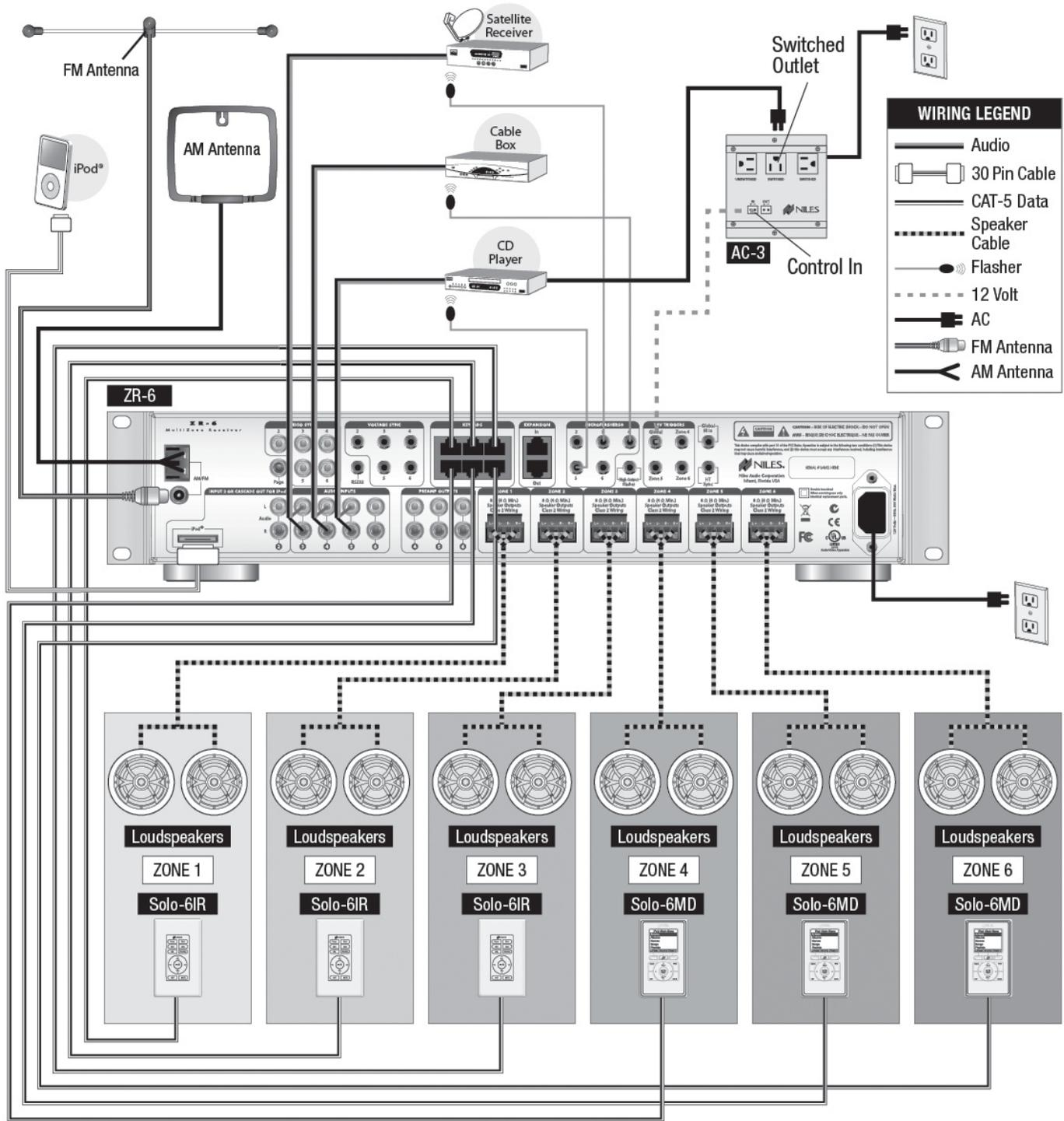
Figure 3. Stand-Alone ZR-6 MultiZone Receiver
