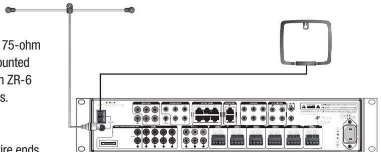
**Figure 15.** Connecting AM/FM Antennas to the ZR-6 MultiZone Receiver
