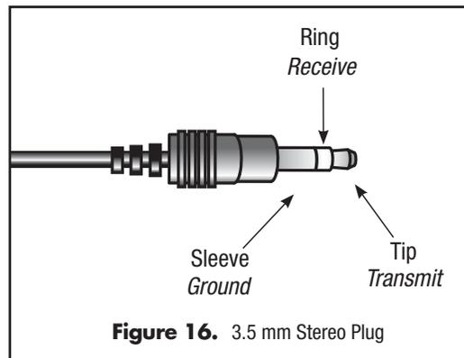
**Figure 16.** 3.5 mm Stereo Plug
