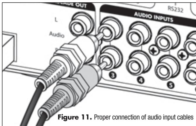
**Figure 11.** Proper connection of audio input cables
