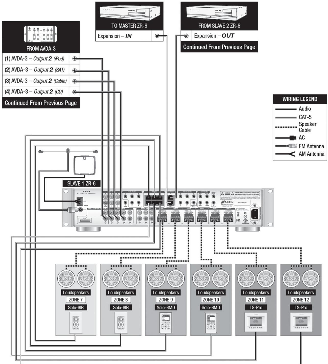
Figure 5b. Expanding to 18 zones. Slave #1 ZR-6 detailed
