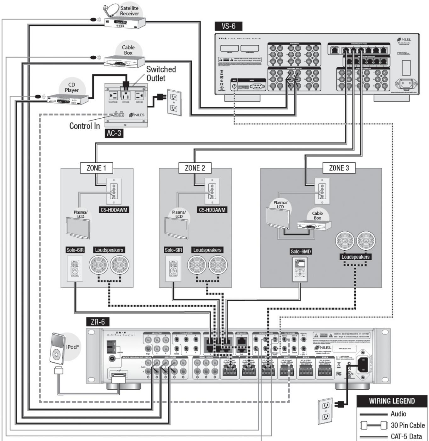
**Figure 4.** Adding a VS-6 for video distribution
