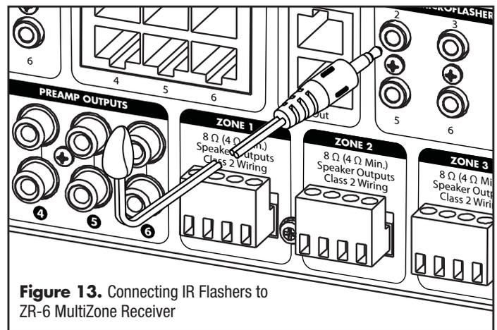
**Figure 13.** Connecting IR Flashers to ZR-6 MultiZone Receiver
