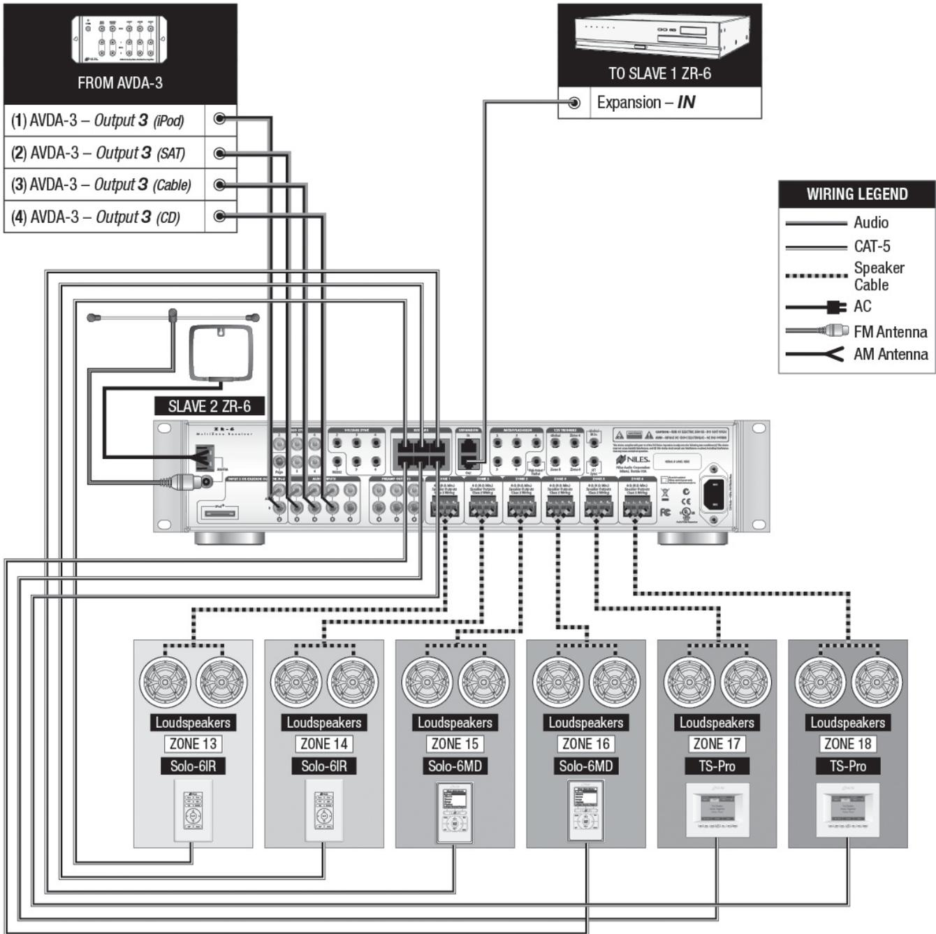
Figure 5c. Expanding to 18 zones. Slave #2 ZR-6 detailed
