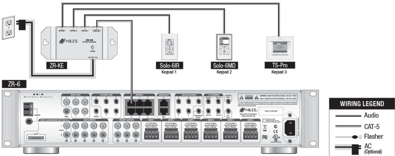
Figure 8. ZR-6 MultiZone Receiver with 3 keypads in zone
