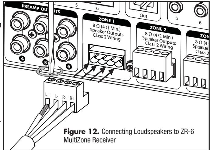
**Figure 12.** Connecting Loudspeakers to ZR-6 MultiZone Receiver
