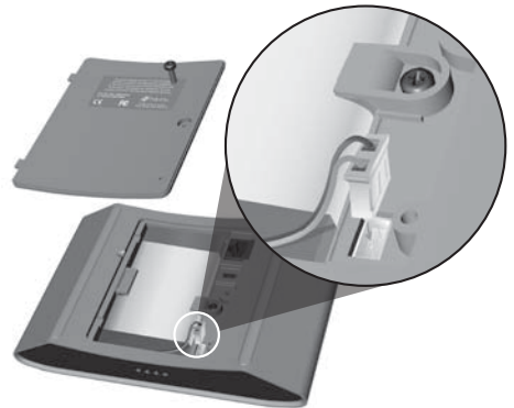
Figure 3: Connecting the iRemoteTS Battery
